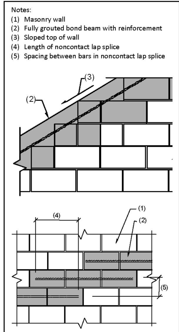
Figure 3 - Examples of a sloped bond beam and a stepped bond beam within a masonry assembly.
