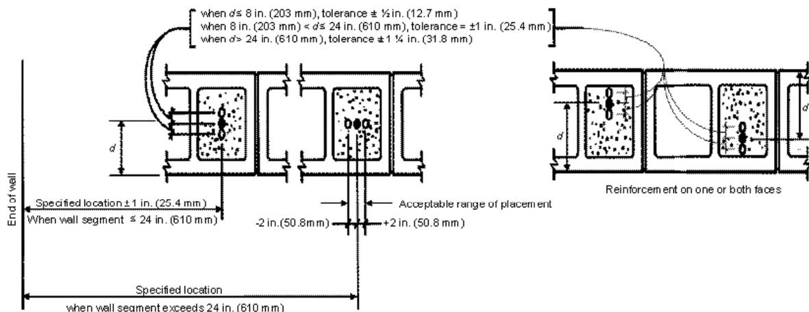
Figure 2 - Placement tolerances for reinforcement embedded in masonry construction based on the effective depth,  $d$ .
